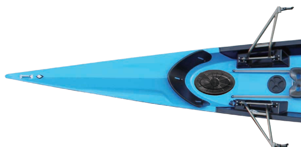
CO4x+ sliding type wave break & choice of hatch
